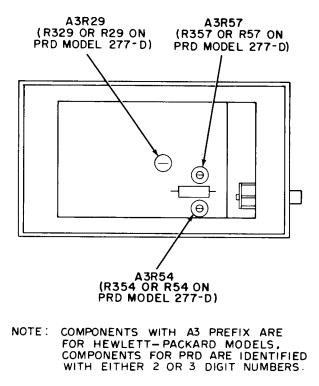
Figure 1. Standing wave ratio meter - left view.
